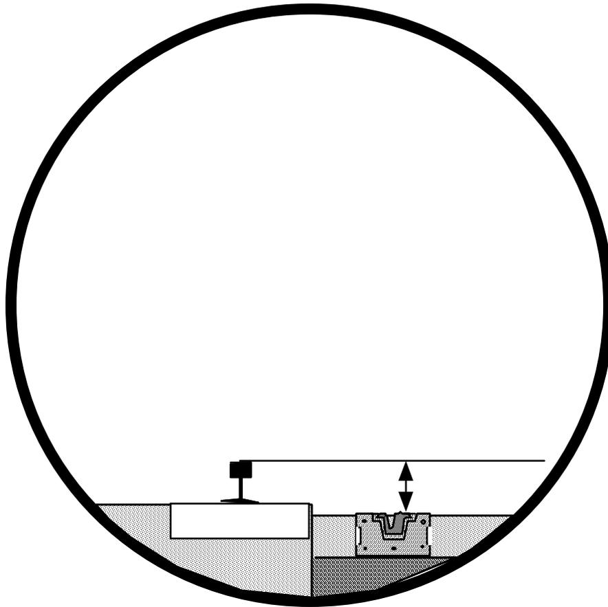
LR55 can also be used for large areas shared between road and rail vehicles like docksides, road/rail freight interchanges, where the shallow depth of the LR55 is compatible with a concrete pavement suitable for heavy goods vehicles.
