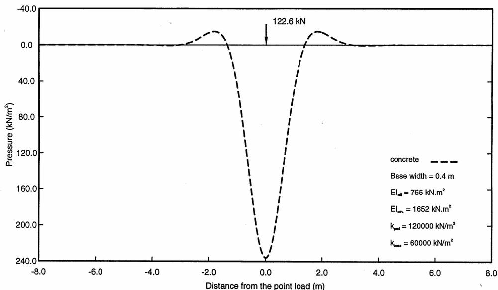
Fig. (1): Pressure distribution on the base of the track due to single wheel of 122.6 kN.
