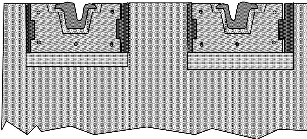
Troughs are laid in advance of the rails and temporarily plated over until the rails are ready to install. By this means a complete installation of four rails for a double track can be completed at the rate of about 400m or more per week. By the use of several track installation teams a 20km route can be completed in less than 6 months, if there are no road traffic management issues.
